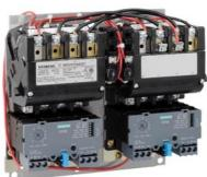
2-speed 3-phase motor starter Size 2 One winding consequent pole Constant or variable torque Solid-state overload relays Low SPD OLR range 13-52a High SPD OLR range 13-52a 110-120/220-240VAC 60HZ coil Enclosure NEMA type (open) No enclosure
