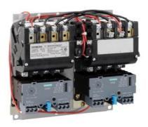
2-speed 3-phase motor starter Size 1 3/4 Two separate windings Constant or variable torque Solid-state overload relays Low SPD OLR range 10-40a High SPD OLR range 10-40a 110V 50HZ / 120V 60HZ coil Enclosure NEMA type (open) No enclosure
