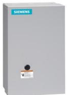
2-speed 3-phase motor starter Size 1 One winding consequent pole Constant or variable torque Solid-state overload relays Low SPD OLR range 5.5-22A High SPD OLR range 10-40a 110-120/220-240VAC 60HZ coil Enclosure NEMA type 1 Indoor general purpose use
