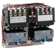
2-speed 3-phase motor starter Size 1 One winding consequent pole Constant or variable torque Solid-state overload relays Low SPD OLR range 3-12A High SPD OLR range 3-12A 110-120/220-240VAC 60HZ coil Enclosure NEMA type (open) No enclosure
