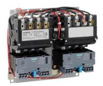
2-speed 3-phase motor starter Size 0 Two separate windings Constant or variable torque Solid-state overload relays Low SPD OLR range 3-12A High SPD OLR range 3-12A 110V 50HZ / 120V 60HZ coil Enclosure NEMA type (open) No enclosure
