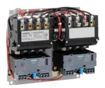
2-speed 3-phase motor starter Size 0 Two separate windings Constant or variable torque Solid-state overload relays Low SPD OLR range 0.75-3.4A High SPD OLR range 3-12A 110V 50HZ / 120V 60HZ coil Enclosure NEMA type (open) No enclosure
