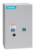
2-speed 3-phase motor starter, Size 0, Two separate windings, Constant or variable torque, Solid-state overload relays, Low Spd OLR range 0.75-3.4A, High Spd OLR range 0.75-3.4A, Enclosure NEMA type 1, Indoor general purpose use
