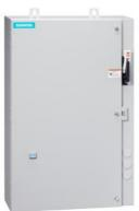
Reversing motor starter, Size 2, Three phase full voltage, Solid-state overload relay, OLR amp range 13-52A, Combination type, 50A circuit breaker, Enclosure NEMA type 4/12, Water/dust tight for outdoors
