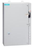
Reversing motor starter, Size 2, Three phase full voltage, Solid-state overload relay, OLR amp range 13-52A, Combination type, 50A circuit breaker, Enclosure NEMA type 4/12, Water/dust tight for outdoors
