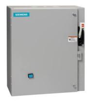
Reversing motor starter, Size 1, Three phase full voltage, Solid-state overload relay, OLR amp range 3-12A, 24VAC 50-60Hz coil, Combination type, 10A circuit breaker, Enclosure NEMA type 1, Indoor general purpose use
