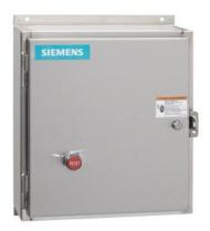
Reversing motor starter, Size 3, Three phase full voltage, Solid-state overload relay, OLR amp range 25-100A, 110V 50Hz / 120V 60Hz coil, Non-combination type, Encl. type 4X 304 S. Steel, Water/dust tight noncorrosive, Standard width enclosure
