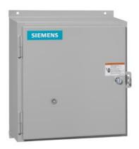
Reversing motor starter, Size 3, Three phase full voltage, Solid-state overload relay, OLRelay amp range 25-100A, 190 220/220 240V 50/60HZ coil, Noncombination type, Enclosure type 4X Fiberglass, Water/dust tight noncorrosive, Standard width enclosure
