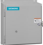
Reversing motor starter, Size 3, Three phase full voltage, Solid-state overload relay, OLR amp range 25-100A, Non-combination type, Enclosure type 4X fiberglass, Water/dust tight noncorrosive, Standard width enclosure
