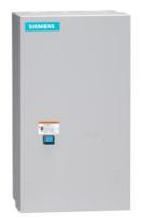
Reversing motor starter, Size 3, Three phase full voltage, Solid-state overload relay, OLR amp range 25-100A, Non-combination type, Enclosure type 1, Indoor general purpose use, Standard width enclosure
