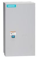
Reversing motor starter, Size 3, Three phase full voltage, Solid-state overload relay, OLR amp range 25-100A, Non-combination type, Enclosure type 1, Indoor general purpose use, Standard width enclosure
