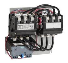
Reversing motor starter Size 3 Three phase full voltage Solid-state overload relay OLRelay amp range 25-100A 110VAC 50HZ / 120VAC 60HZ coil Non-combination type Enclosure type (open)
