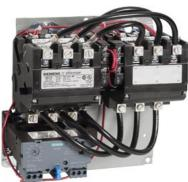
Reversing motor starter Size 3 Three phase full voltage Solid-state overload relay OLRelay amp range 25-100A 208VAC 60HZ coil Non-combination type Enclosure type (open)
