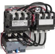
Reversing motor starter Size 3 Three phase full voltage Solid-state overload relay OLRelay amp range 25-100A 220-240/440-480VAC 60HZ coil Non-combination type Enclosure type (open)
