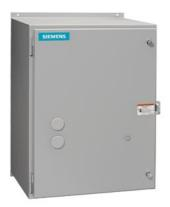
Reversing motor starter, Size 3, Three phase full voltage, Solid-state overload relay, OLRelay amp range 25-100A, 380 440/440 480V 50/60HZ coil, Noncombination type, Enclosure type 12, Dust/drip proof for indoors, Standard width enclosure
