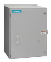
Reversing motor starter, Size 3, Three phase full voltage, Solid-state overload relay, OLR amp range 25-100A, Non-combination type, Enclosure type 12, Dust/drip proof for indoors, Standard width enclosure
