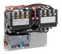
Reversing motor starter Size 2 Three phase full voltage Solid-state overload relay OLRelay amp range 13-52a 380-440/440-480V 50/60HZ coil Non-combination type Enclosure type (open)
