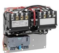
Reversing motor starter Size 1 Three phase full voltage Solid-state overload relay OLRelay amp range 10-40a 110VAC 50HZ / 120VAC 60HZ coil Non-combination type Enclosure type (open)
