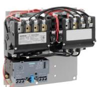
Reversing motor starter Size 1 Three phase full voltage Solid-state overload relay OLRelay amp range 3-12A 380-440/440-480V 50/60HZ coil Non-combination type Enclosure type (open)
