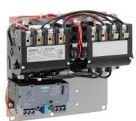
Reversing motor starter Size 0 Three phase full voltage Solid-state overload relay OLRelay amp range 3-12A 380-440/440-480V 50/60HZ coil Non-combination type Enclosure type (open)
