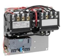
Reversing motor starter, Size 00, Three phase full voltage, Solid-state overload relay, OLRelay amp range 3-12a, 190 220/220 240V 50/60HZ coil, Non-combination type, Enclosure type (open), No enclosure
