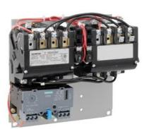
Reversing motor starter, Size 00, Three phase full voltage, Solid-state overload relay, OLRelay amp range 3-12a, 220 240/440 480VAC 60HZ coil, Non-combination type, Enclosure type (open), No enclosure
