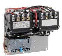
Reversing motor starter, Size 00, Three phase full voltage, Solid-state overload relay, OLRelay amp range 0.25-1a, 380 440/440 480V 50/60HZ coil, Non-combination type, Enclosure type (open), No enclosure
