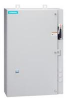
Non-reversing motor starter, Size 2, Three phase full voltage, Solid-state overload relay, OLR amp range 13-52A, 110V 50Hz / 120V 60Hz coil, Combination type, 50A circuit breaker, Enclosure NEMA type 4/12, Water/dust tight for outdoors, Extra-wide enclosure
