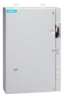
Non-reversing motor starter, Size 4, Three phase full voltage, Solid-state overload relay, OLR amp range 50-200A, Combination type, 200A non-fusible disconnect, Enclosure NEMA type 4/12, Water/dust tight for outdoors, Standard width enclosure
