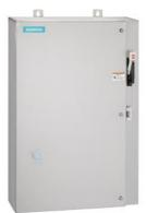
Non-reversing motor starter Size 3 Three phase full voltage Solid-state overload relay OLRelay amp range 25-100A 240VAC 50HZ / 277VAC 60HZ coil Combination type 200A fusible disconnect 200A/250V fuse clip Encl NEMA type 4X 316 S-steel Water/dust tight non-corrosive Standard width enclosure
