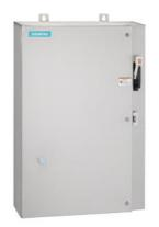
Non-reversing motor starter, Size 3, Three phase full voltage, Solid-state overload relay, OLR amp range 25-100A, Combination type, 200A fusible disconnect, 200A/250V fuse clip, Encl NEMA type 4X 304 S-Steel, Water/dust tight noncorrosive, Standard width enclosure
