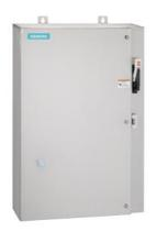
Non-reversing motor starter, Size 3, Three phase full voltage, Solid-state overload relay, OLR amp range 25-100A, 110V 50Hz / 120V 60Hz coil, Combination type, 200A fusible disconnect, 200A/250V fuse clip, Encl NEMA type 4X 304 S-Steel, Water/dust tight noncorrosive, Standard width enclosure
