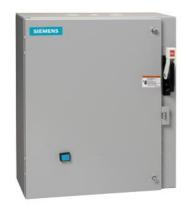
Non-reversing motor starter Size 3 Three phase full voltage Solid-state overload relay OLRelay amp range 25-100A 380-440/440-480V 50/60HZ coil Combination type 100A fusible disconnect 100A/250V fuse clip Enclosure NEMA type 1 Indoor general purpose use Standard width enclosure
