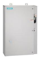
Non-reversing motor starter Size 3 Three phase full voltage Solid-state overload relay OLRelay amp range 25-100A 24Vdc coil Combination type 100A non-fusible disconnect Encl NEMA type 4X 304 S-steel Water/dust tight non-corrosive Extrawide enclosure
