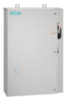
Non-reversing motor starter Size 3 Three phase full voltage Solid-state overload relay OLRelay amp range 25-100A 24Vdc coil Combination type 100A fusible disconnect 100A/250V fuse clip Encl NEMA type 4X 304 S-steel Water/dust tight non-corrosive Extra-wide enclosure
