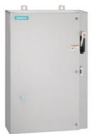
Non-reversing motor starter, Size 3, Three phase full voltage, Solid-state overload relay, OLR amp range 25-100A, Combination type, 200A fusible disconnect, 200A/250V fuse clip, Encl NEMA type 4X 304 S-Steel, Water/dust tight noncorrosive, Extra-wide enclosure
