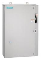
Non-reversing motor starter, Size 3, Three phase full voltage, Solid-state overload relay, OLR amp range 25-100A, Combination type, 100A fusible disconnect, 100A/600V fuse clip, Encl NEMA type 4X 304 S-Steel, Water/dust tight noncorrosive, Extra-wide enclosure
