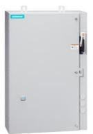
Non-reversing motor starter, Size 3, Three phase full voltage, Solid-state overload relay, OLR amp range 25-100A, Combination type, 100A fusible disconnect, 100A/600V fuse clip, Enclosure NEMA type 4/12, Water/dust tight for outdoors, Extra-wide enclosure
