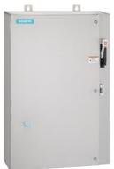
Non-reversing motor starter, Size 2 1/2, Three phase full voltage, Solid-state overload relay, OLR amp range 25-100A, Combination type, 100A fusible disconnect, 100A/250V fuse clip, Encl NEMA type 4X 304 S-Steel, Water/dust tight noncorrosive, Extra-wide enclosure
