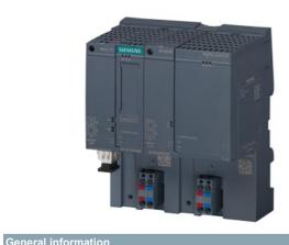
SIMATIC PN/PN Coupler for deterministic data exchange between max.4 PN-Controller per subnet, also from subnet to subnet, PROFIsafe data exchange, I/O-, MSI-, MSO- and data record communication, redundant power supply, PN-connection via SIMATIC BusAdapter (BA), delivery w/o BusAdapter
