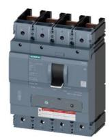
circuit breaker 3VA5 UL frame 400 breaking capacity class C 100kA @ 480 V 4-pole, line protection TM240, ATAM, In=400A overload protection Ir=280A ...400A short circuit protection Ii=5...10 x In neutral unprotected w/o connection
