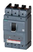
circuit breaker 3VA5 UL frame 400 breaking capacity class C 100kA @ 480 V 3-pole, line protection TM240, ATAM, In=400A overload protection Ir=280A ...400A short circuit protection Ii=5...10 x In w/o connection
