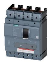
circuit breaker 3VA5 UL frame 400 breaking capacity class C 100kA @ 480 V 4-pole, line protection TM230, FTAM, In=400A overload protection Ir=400A fixed short circuit protection li=5...10 x In neutral unprotected w/o connection
