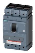
circuit breaker 3VA5 UL frame 400 breaking capacity class C 100kA @ 480 V 3-pole, line protection TM230, FTAM, In=400A overload protection Ir=400A fixed short circuit protection Ii=5...10 x In Al-lug, line and load side
