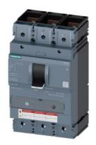
circuit breaker 3VA5 UL frame 400 breaking capacity class C 100kA @ 480 V 3-pole, line protection TM230, FTAM, In=400A overload protection Ir=400A fixed short circuit protection li=5...10 x In nut keeper kit on both sides
