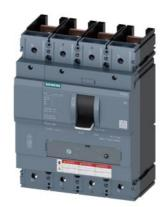
circuit breaker 3VA5 UL frame 400 breaking capacity class H 65kA @ 480 V 4-pole, line protection TM230, FTAM, In=400A without overload protection Ir=400A fixed short circuit protection Ii=5...10 x In neutral protection 1 w/o connection
