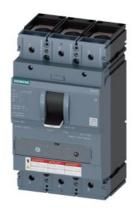
circuit breaker 3VA5 UL frame 400 breaking capacity class H 65kA @ 480 V 3-pole, line protection TM240, ATAM, In=400A overload protection Ir=320A ...400A short circuit protection Ii=5...10 x In Al-lug, line and load side
