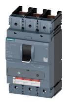
circuit breaker 3VA5 UL frame 400 breaking capacity class M 35kA @ 480 V 3-pole, line protection TM240, ATAM, In=400A without overload protection Ir=280A ...400A short circuit protection Ii=5...10 x In w/o connection
