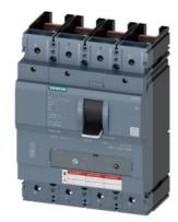
circuit breaker 3VA5 UL frame 400 breaking capacity class C 100kA @ 480 V 4-pole, line protection TM230, FTAM, In=350A overload protection Ir=350A fixed short circuit protection li=5...10 x In neutral unprotected w/o connection
