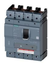
circuit breaker 3VA5 UL frame 400 breaking capacity class H 65kA @ 480 V 4-pole, line protection TM230, FTAM, In=350A without overload protection Ir=350A fixed short circuit protection Ii=5...10 x In neutral protection 1 w/o connection
